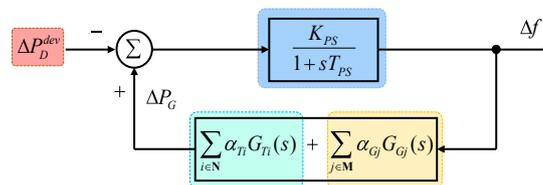
(b) The simplified power system transfer function model.
