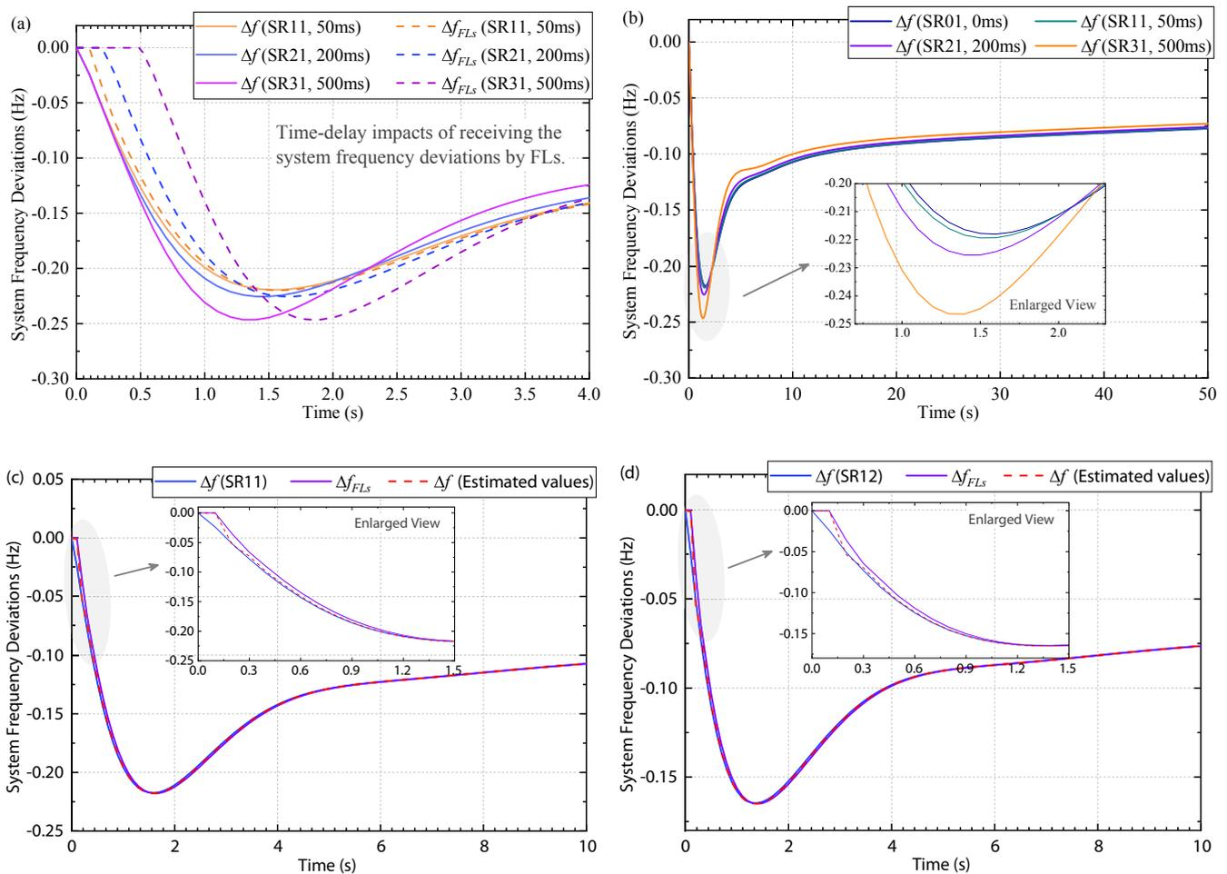
**Fig. 15.** The communication time-delay impacts and correction results of frequency deviations by utilizing the proposed adaptive time-delay control scheme. (a) Communication time-delay impacts on frequency detections in SR11, SR21, and SR31; (b) Comparisons of frequency deviations in SR01, SR11, SR21, and SR31; (c) The actual, FL-receiving and corrected frequency deviations in SR11; (d) The actual, FL-receiving and corrected frequency deviations in SR12.
