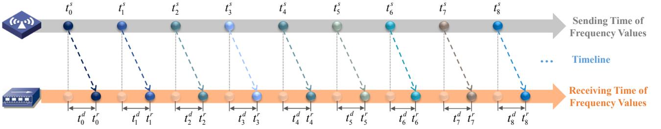
Fig. 6. Communication delay in the control process of flexible loads.
