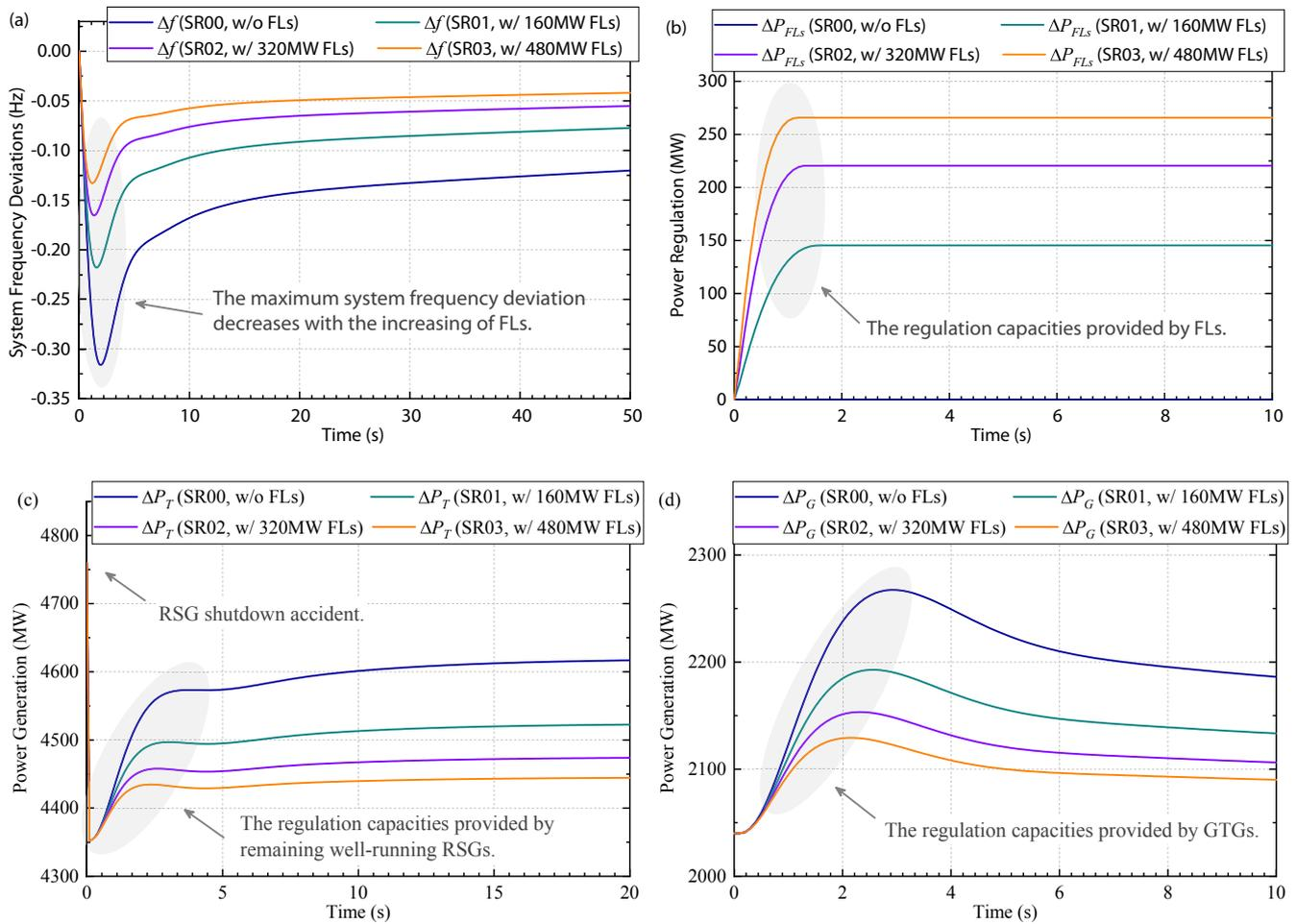
**Fig. 14.** The frequency deviations of the power system and the regulation power from FLs, RSGs and GTGs in SR00, SR01, SR02, and SR03. (a) Frequency deviation comparisons of the power system; (b) Regulation power comparisons provided by FLs; (c) Shutdown accident and regulation power of RSGs; (d) Regulation power comparisons provided by GTGs.
