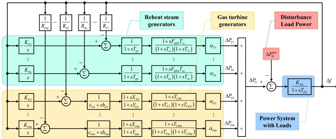
(a) The detailed power system transfer function model.
