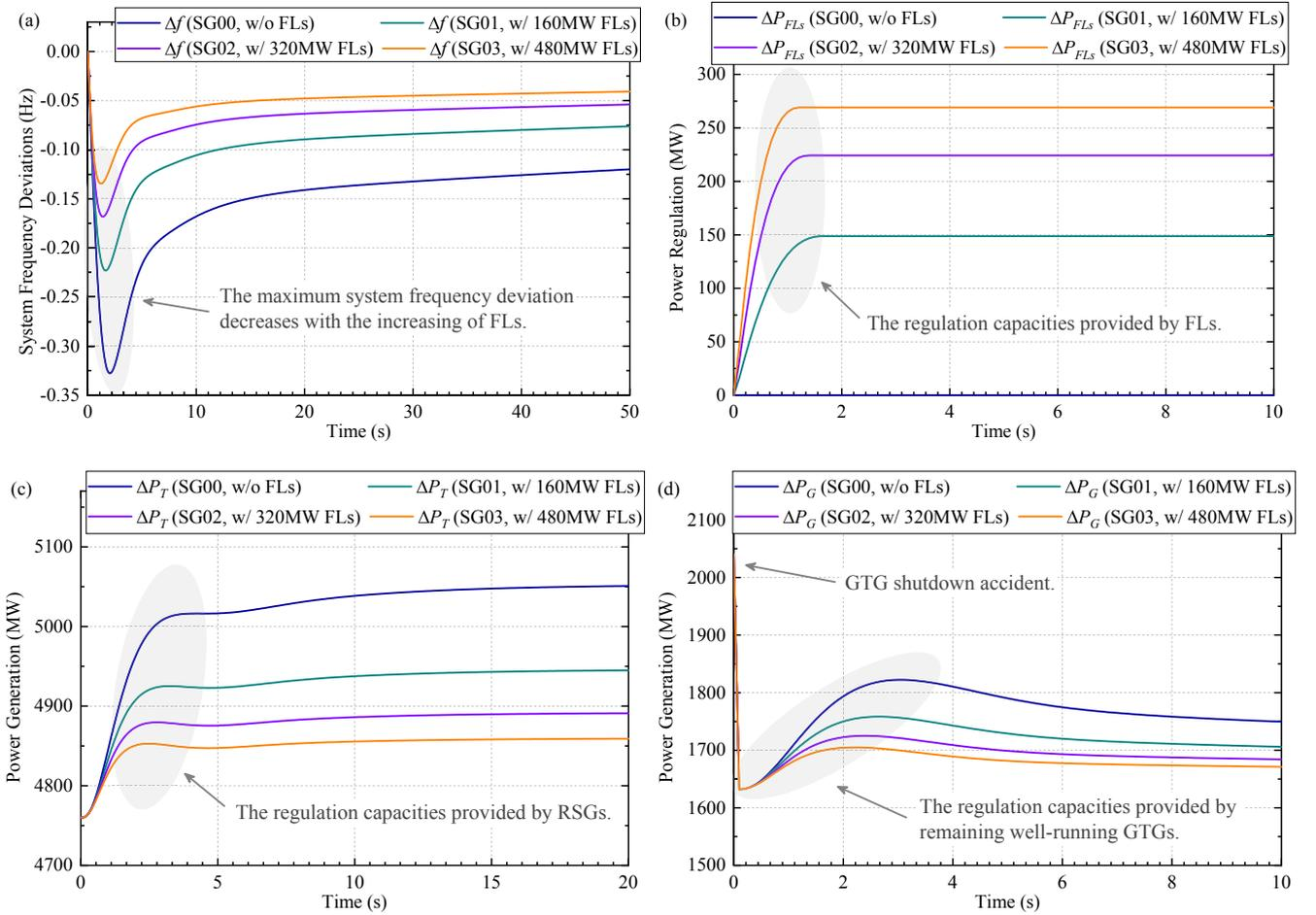
**Fig. 11.** The frequency deviations of the power system and the regulation power from FLs, RSGs and GTGs, in cases SG00, SG01, SG02, and SG03. (a) Frequency deviation comparisons of the power system; (b) Regulation power comparisons provided by FLs; (c) Regulation power comparisons provided by RSGs; (d) Shutdown accident and regulation power of GTGs.
