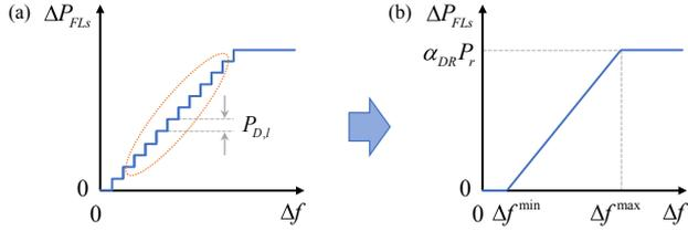
Fig. 4. The regulation power provided by flexible loads utilizing the on-off control method. (a) The micro curve of the regulation power provided by each flexible load. (b) The macro curve of the regulation power provided by large-scale flexible loads.
