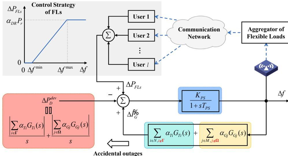
Fig. 5. The reconstructed transfer function model of the power system with reheat steam generators and gas turbine generators after accidental outages of generating units, considering the frequency regulation of flexible loads.
