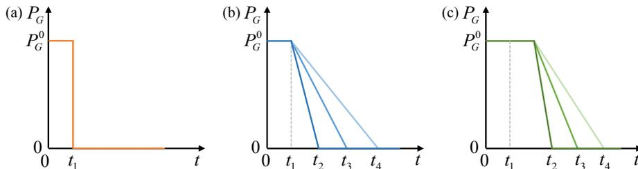
Fig. 2. The distinctions among three typical outages in power systems. (a) The accidental outage. (b) The slow-changing outages. (c) The lagging outages.
