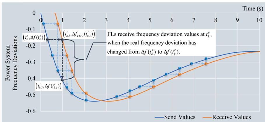
Fig. 8. The sent and received system frequency deviations for flexible loads when participating in power systems' regulation services.
