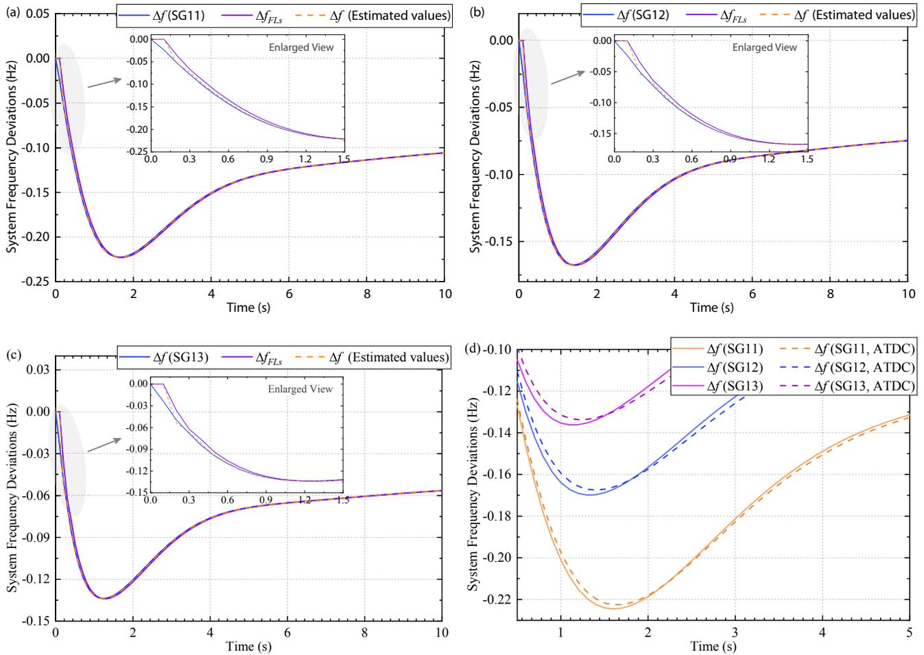
**Fig. 13.** The correction results of frequency deviations by utilizing the proposed adaptive time-delay control scheme. (a) The actual, FL-receiving and corrected frequency deviations in SG11; (b) The actual, FL-receiving and corrected frequency deviations in SG12; (c) The actual, FL-receiving and corrected frequency deviations in SG13; (d) The frequency deviation comparisons before and after correction by utilizing the proposed adaptive time-delay control scheme in SG11, SG12 and SG13.
