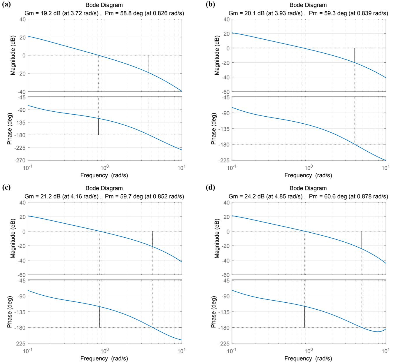
**Fig. 10.** The Bode plot comparisons of the power system with and without FLS when the communication delay is not considered during the control process of FLS. (a) SG00, without FLS; (b) SG01, with 160 MW FLS for providing regulation services; (c) SG02, with 320 MW FLS for providing regulation services; (d) SG03, with 480 MW FLS for providing regulation services.
