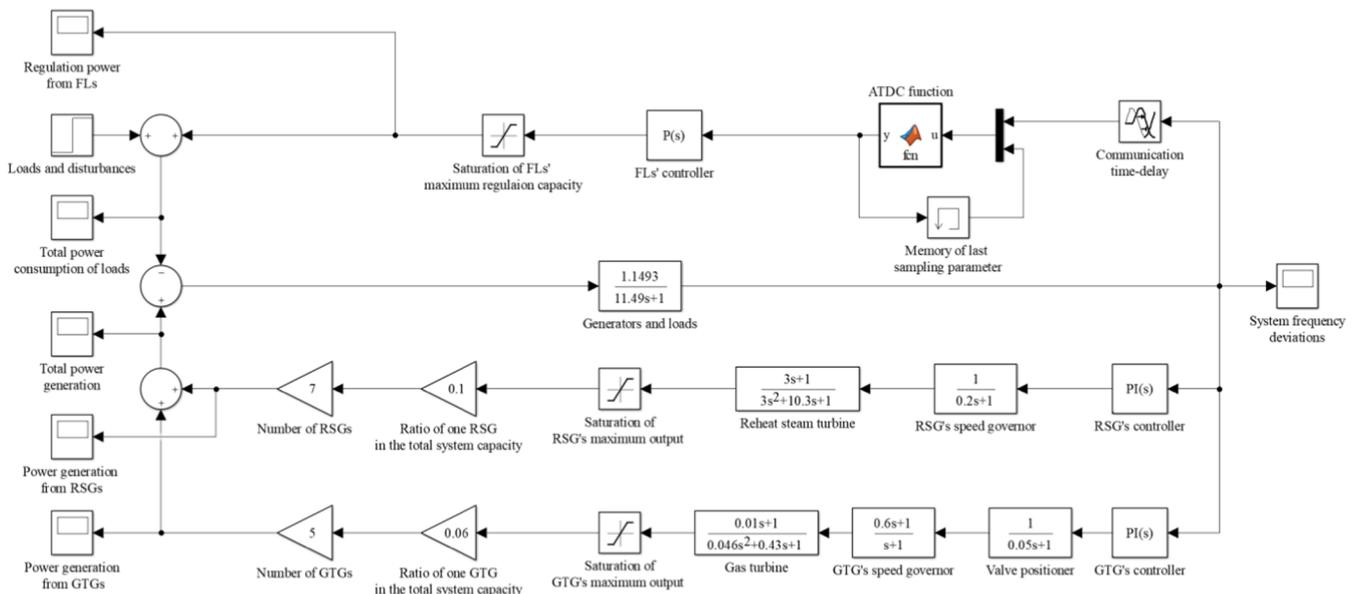
Fig. 16. Simulink model of the adaptive time-delay control of flexible loads in the test system.
