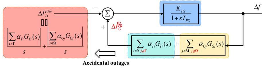
Fig. 3. The reconstructed transfer function model of the power system with reheat steam generators and gas turbine generators after accidental outages of generating units.
