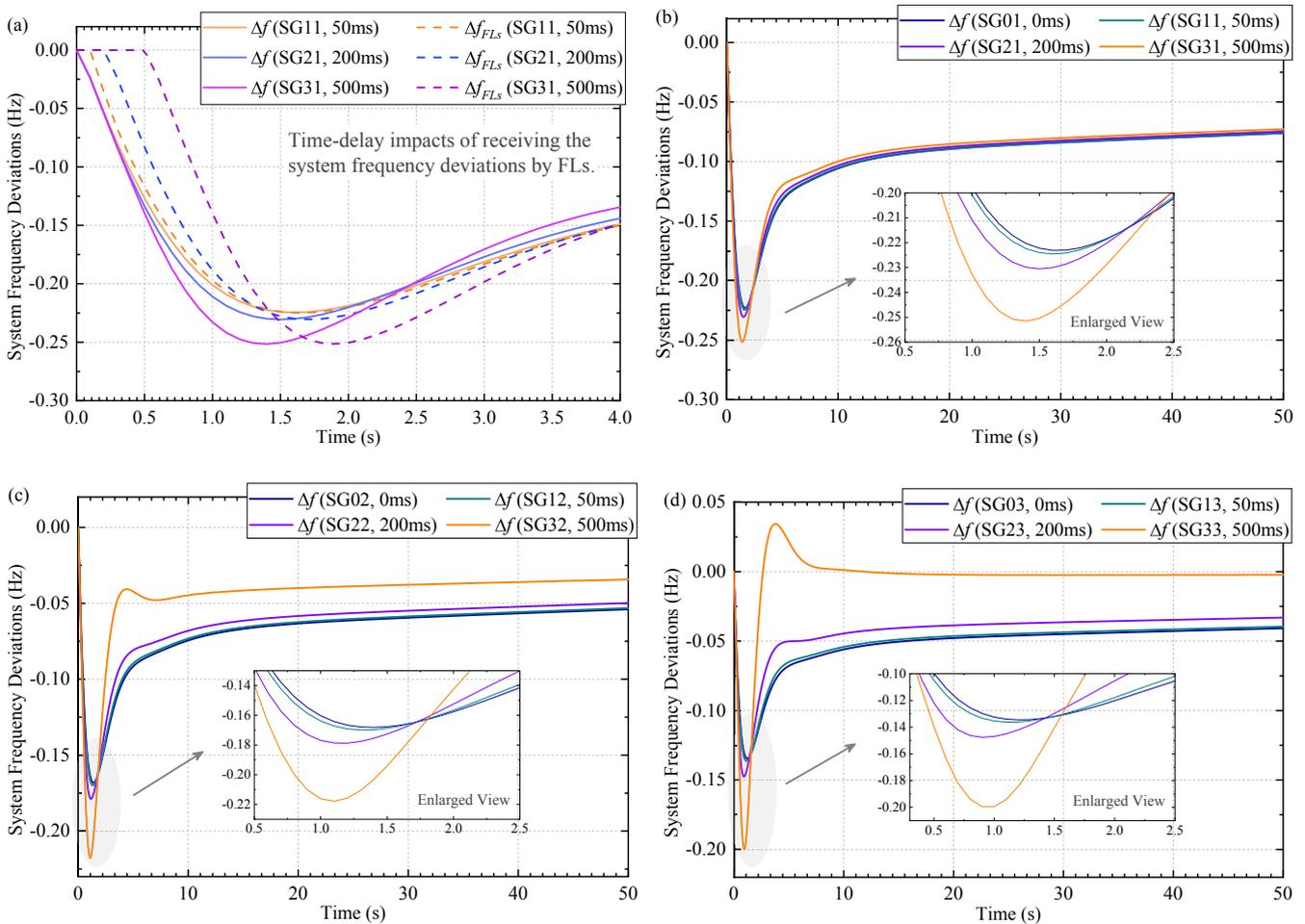
**Fig. 12.** The power system frequency deviations caused by different communication time-delay, including 0 ms, 50 ms, 200 ms, and 500 ms. (a) Communication time-delay impacts on frequency detections in SG11, SG21, and SG31; (b) Comparisons of frequency deviations in SG01, SG11, SG21, and SG31; (c) Comparisons of frequency deviations in SG02, SG12, SG22, and SG32; (d) Comparisons of frequency deviations in SG03, SG13, SG23, and SG33.
