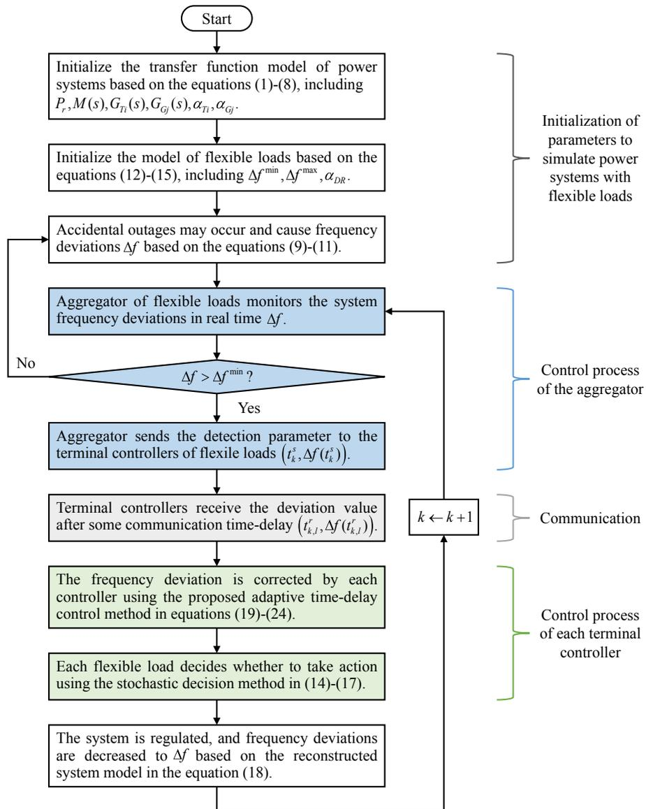
**Fig. 9.** The implementation procedure of the adaptive time-delay control of flexible loads.
