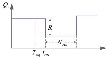
Fig. 3. Response characteristics to incentive signal.
