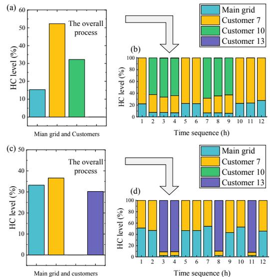
Fig. 13. Comparison of evaluations under different time-scales for 7-th harmonic (a) the overall process (half of a day); (b) hourly; and 13-th harmonic (c) the overall process (half of a day); (d) hourly.
