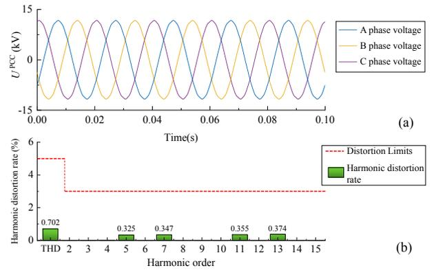
Fig. 16. The voltage at the PCC under the second suppression scheme based on the proposed method (a) time-domain three-phase waveform; (b) frequency-domain harmonic distortion rate.
