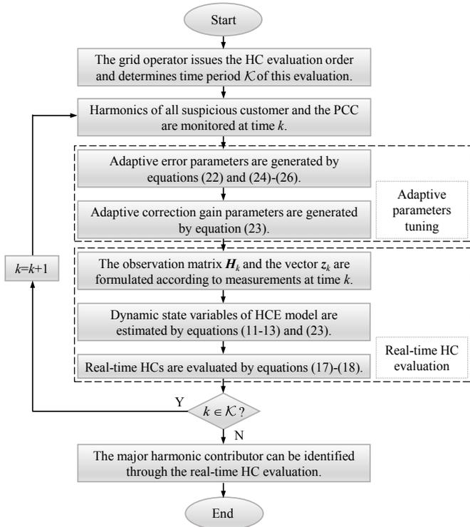
Fig. 6. The procedure of real-time HC evaluation method.
