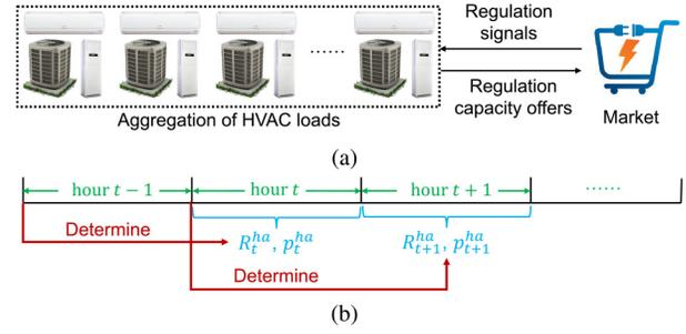
Fig. 1. (a) System configuration of scheduling HVAC systems to provide regulation services and (b) schema of hour-ahead regulation capacity offers in the PJM market.
